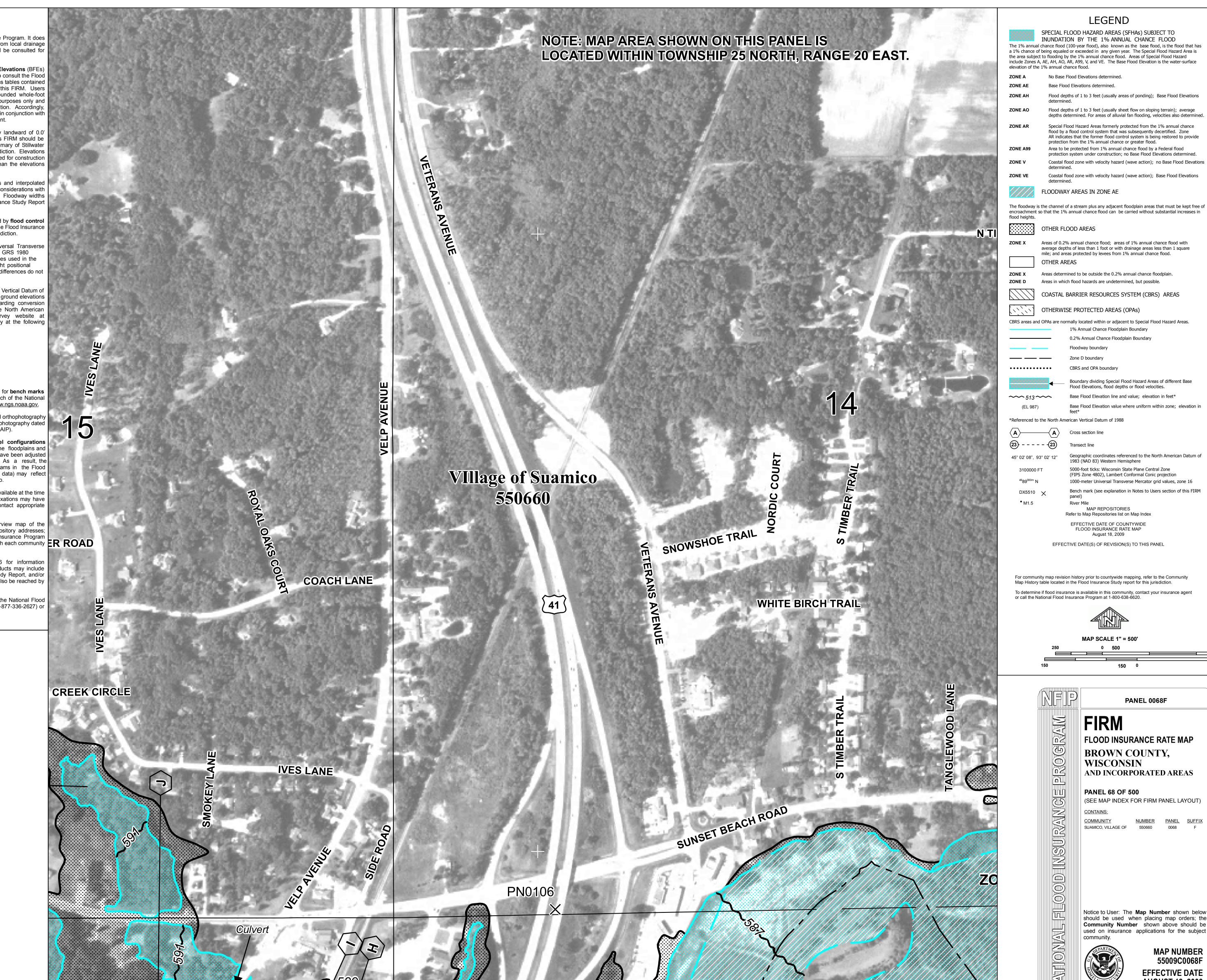
The 1% annual chance flood (100-year flood), also known as the base flood, is the flood that has a 1% chance of being equaled or exceeded in any given year. The Special Flood Hazard Area is
